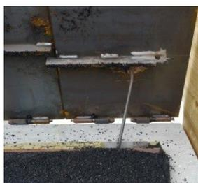
The environmental Bullet Catcher is filled with ricochet and fire retardant rubber granulate.
